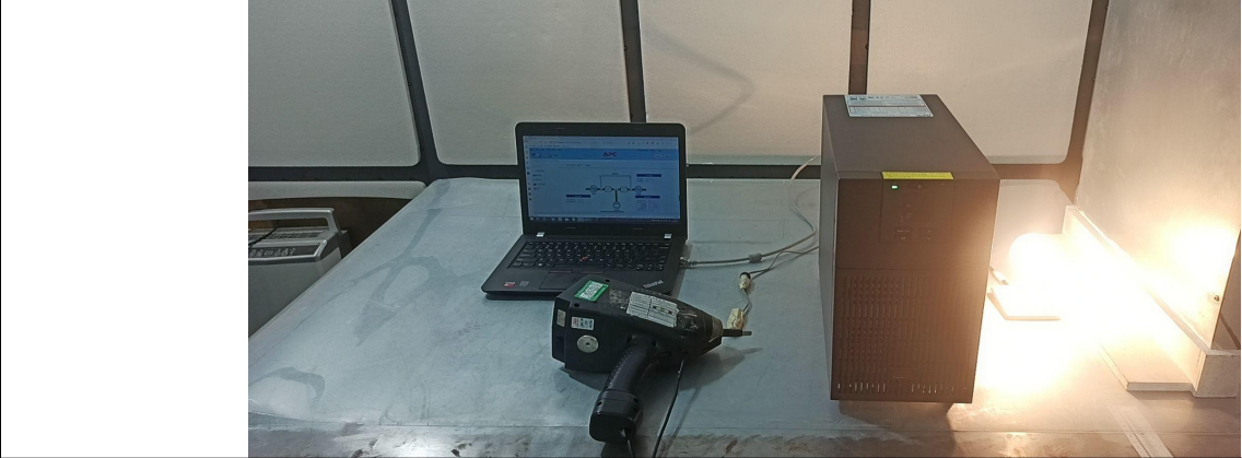
Set-up for Magnetic Field Immunity
